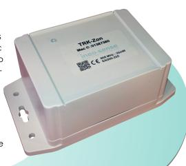
Thanks to Clover-Net® power-consumption optimization, it can run on a simple battery. For intensive usage, it can either embedded a second battery or have external power supply (with battery backup).
